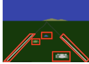
Figure 3: An example of object detection in car driving game Enduro. Users were allowed to remove or add other bounding regions at will.
